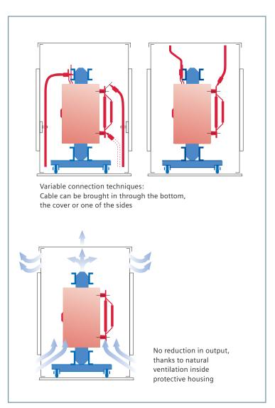
Design of housing cover, degree of protection IP 23 (indoor installation)
